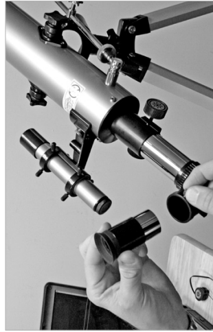
Fig. 10: Remove the eyepiece from the telescope.
